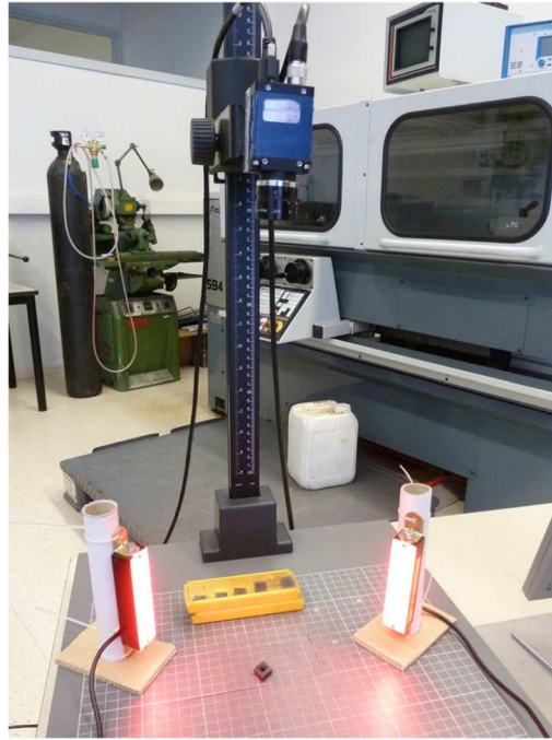
Figure 61. Image capture prototype. The support in which the camera is placed and the LED bars employed are shown [136].
