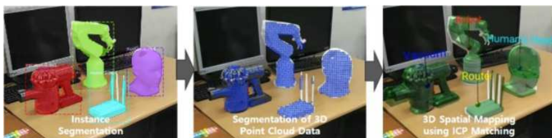
Figure 67. Demonstration of the deep learning-based 3D spatial mapping [152].
