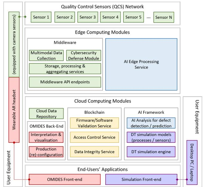
Fig. 1. OPTIMAI generic service-oriented functional architecture for ZDM. Color-coding is used to identify technologies as belonging to an emerging topic in smart manufacturing (green for multi-sensory data acquisition; blue for AI analysis; yellow for distributed ledger technologies; red for context-aware AR; and purple for DT-enabled production optimisation inference).
