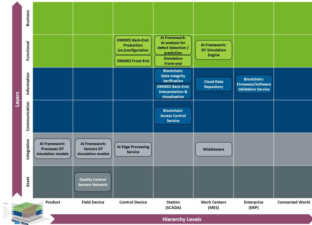
Fig. 3. OPTIMAI Layer-and-Hierarchy mapping to RAMI 4.0.
