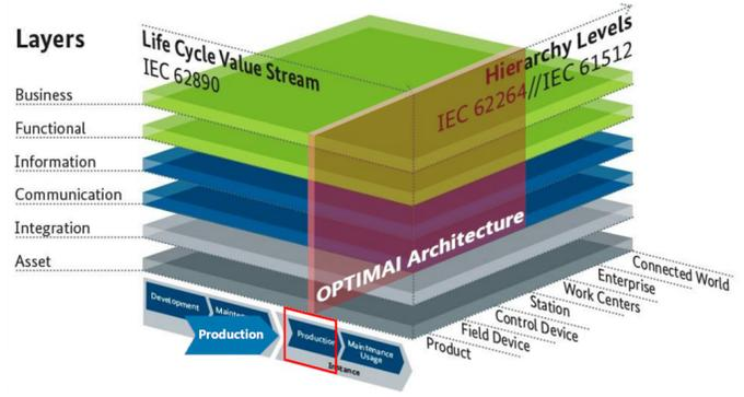
Fig. 2. OPTIMAI RAMI 4.0 "slice" in the 3D RA. Adapted from the original graphic © Plattform Industrie 4.0 and ZVEI, retrieved from [4]
