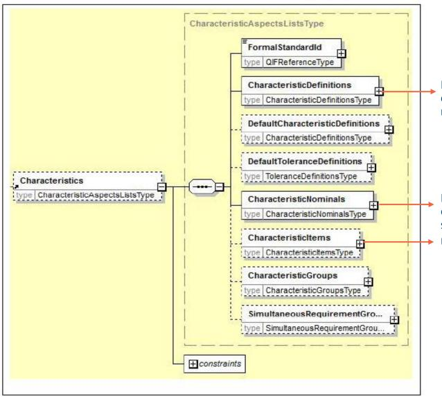
Part of a characteristic that can be shared among different characteristics (e.g. standard diameter tolerance from a manufacturer for a part)
